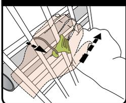
Insert the hook into the loop of the clip, rest the bottom of the Driver against the pole, and lever the clip off whilst covering the clip with your other hand, making it easier to recover.
