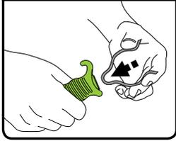
Insert the KwikAz clip into the jaws on the front of the Driver and push down until fully engaged.
