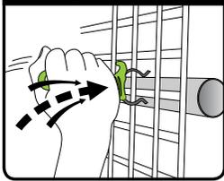
In a single action, firmly strike the KwikAz clip through the containment screening and around the pole/standard. Ensure the clip is perpendicular to the standard or ledger, and not at an angle.
