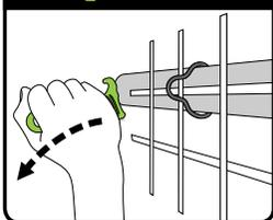
Withdraw the Driver leaving the KwikAz clip attached to the containment screening and the pole/standard.
