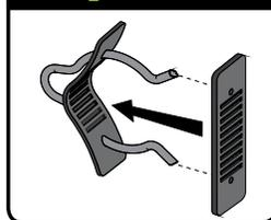
Insert the legs of the clip through the holes in the Gripz with the gripping grooves facing outward.
